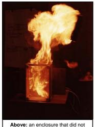
The heart of the Flameproof concept is in providing a strong and closely fitting enclosure to protect its contents. The enclosure must be capable of containing an explosion.
