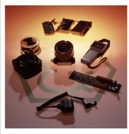
Encapsulation works simply by enclosing equipment in potting compound so keeping the potentially explosive atmosphere away from the source of ignition. There are however, several drawbacks with this type of protection. The testing part of certification the process takes at
